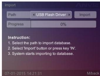
Select the source file directory, press [▼] key to select [Import] button and press [OK] key to import the source data into the system database.
