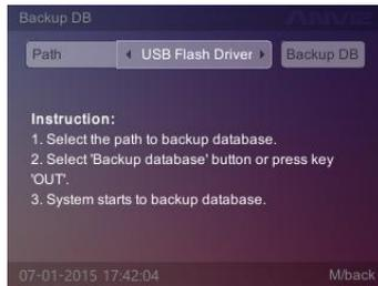
Select path to save the database, then select [Backup DB] button and press [OK] key to backup the database. After backup the system will prompt: “Backup DB completed!”.
