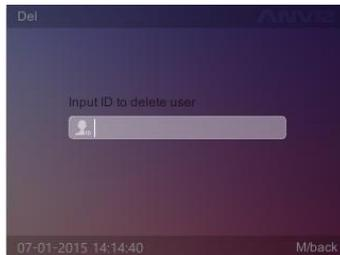
Input ID and press [OK] key to confirm, the system prompts 'Delete User and FP OK!'. Press [OK] key to confirm delete, press [M] key to cancel.
