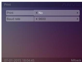
Enable/Disable print function and Baud rate for communication with printer, press “ESC” to save and exit.
