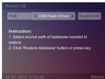
Select the database files, select [Restore DB] button and press [OK] key to restart system.
