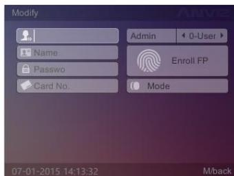
Enter the ID and press [OK] key to confirm, the user information display automatically then could modify the user information. After finished, press [M] key to save the modification for user.
