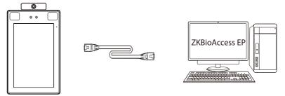
Default IP address: 192.168.1.201 Subnet mask: 255.255.255.0 IP address: 192.168.1.130 Subnet mask: 255.255.255.0
