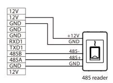
**Note:** 485A and 485B can be connected to the barrier gate or the 485 reader, but cannot be connected to the gate and the reader at the same time.
